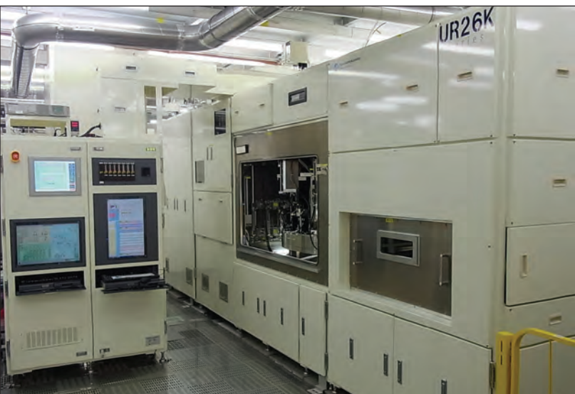
The Taiyo Nippon Sanso UR26K is the company's biggest MOCVD reactor
