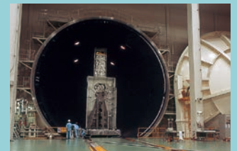
Space simulation chamber
