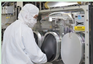
R&D-oriented equipment uses glove boxes for the manual insertion of substrates into the reactor.
