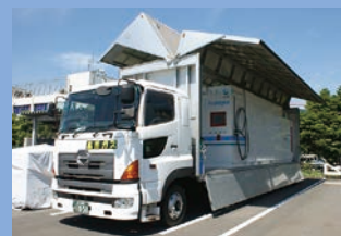
Packaged hydrogen station Hydro Shuttle
